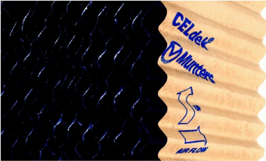
*The air entering face of the pad suffers the most damaging effects of sunlight, algae, dirt, and environmental chemicals. Optional MI-T-edge algae resistant edge coating helps guard against these elements, and can significantly extend the life of the evaporative pad.*
