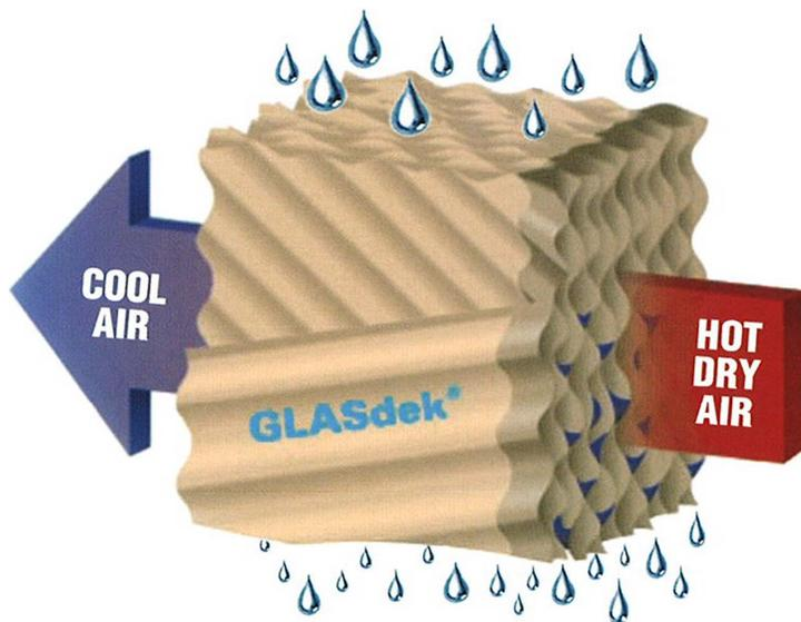
*The shallow angle of Munters unequal flute design allows high velocity air to travel through the pad without significant resistance or water droplet carry over. GLASdek's self-cleaning design resists the clogging caused by dust, sand or other debris. By design, more water is directed toward the air entering face of the pad, where it flushes away dirt and debris.*
