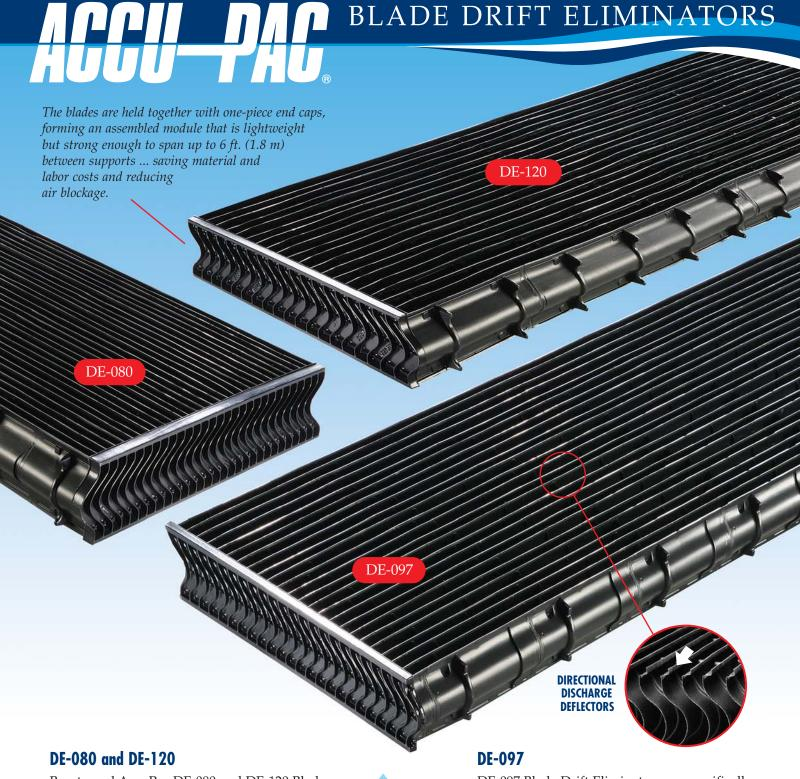
Brentwood AccuPac DE-080 and DE-120 Blade Drift Eliminator modules use a tightly-spaced series of sinusoidal-shaped PVC (or HPVC) blades that force the leaving air to make distinct changes of direction at three impact zones (right), resulting in maximum drift droplet removal. And this performance does not come at the expense of fan energy, as the engineered flow through these high-performance drift eliminators achieves very low pressure drop (see back).
